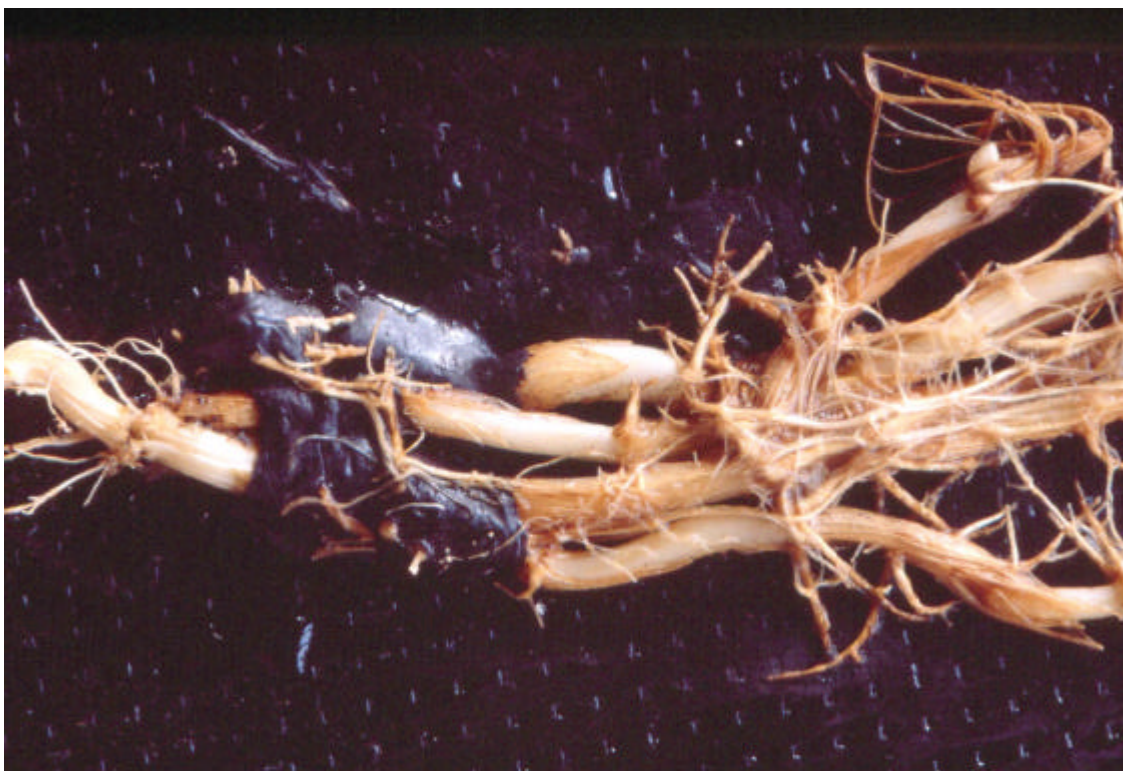
Figure 4: Sheet surface with penetrated rhizomes
