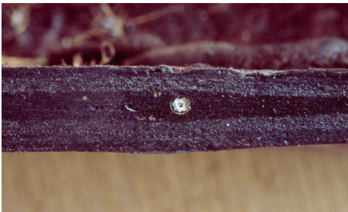
Figure 5: Cut through joint with a penetrated rhizome
