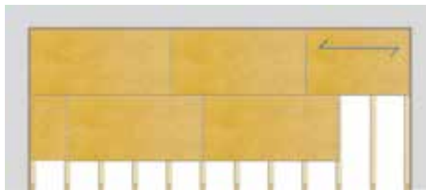
Floating, interlocking installation: Offset 30cm (11.81") Interlocking installation on sleepers: Minimum offset 1 span width
